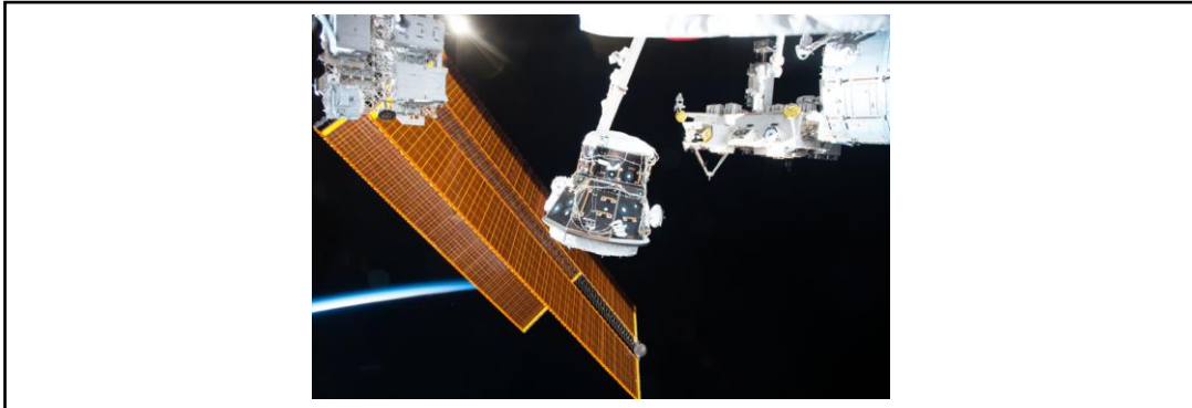
Figure 29 - Attachment of the Pressurized Mating Adapter-3 to the International Space Station using the Canadarm2 robotic arm [21]. Similar procedures in reverse could provide an option for part of the decommissioning.
