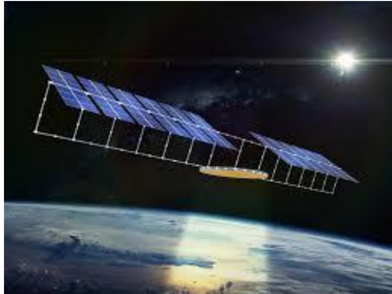
Figure 4 – Rendering of MR-SPS in space showing antenna and panels supported by rotating joints (Xinbin, et al., 2016)
