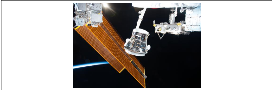
Figure 28 – Attachment of the Pressurized Mating Adapter-3 to the International Space Station using the Canadarm2 robotic arm [21].
