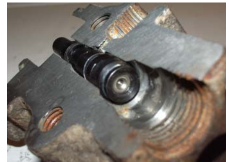
Figure 1: Faulty load sharing valve
