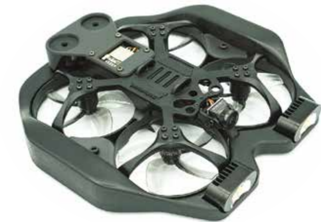
Bespoke prototype UAS with integrated COTS LED dazzler to distract and disorientate a subject at range
